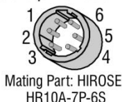
Figure 8: 6-pin Hirose Circular Male Power Plug—Power Connector
