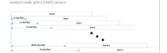
*Line times for the various modes of the Kinetix22 camera.*
