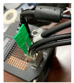
PCIe cables inserted into camera's PCIe ports.
