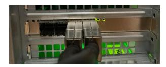
If one or both LEDs are orange instead of green, make sure the cables are connected in the right ports order and are undamaged.
