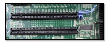
5. Hold the PCIe card (being careful not to touch the board components or PCIe bridge pins) and insert it, properly orientated, into the open slot. The card should slide into place with minimal resistance and click when fully inserted.
