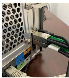
PCIe cables inserted into PCIe interface card's ports.
