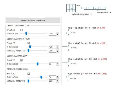
For example, in the figure above, a Despeckle Dark Low threshold of "66" indicates that a pixel that is 34% below the local median will be replaced by the local median. A Despeckle Bright High threshold of "120" indicates that a pixel that is 20% brighter than the local median will be replaced.
