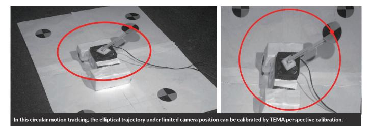
2D tracking is the basic functionality of TEMA. Tracking a marker or an object in the image sequence using any algorithm from the available library will produce 2D pixel coordinates. Those 2D coordinates can then be used to calculate velocity, acceleration, distances and angles. They will also serve for basis when dealing with 3D or 6DoF calculations.
