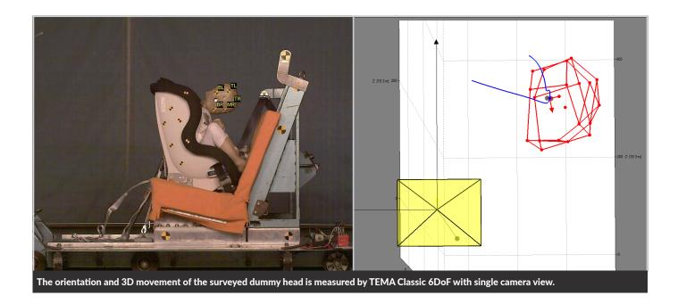
Tracking in 6 degrees of freedom (6DoF) is an optional feature of TEMA that computes the position and orientation of a rigid tracked object.
