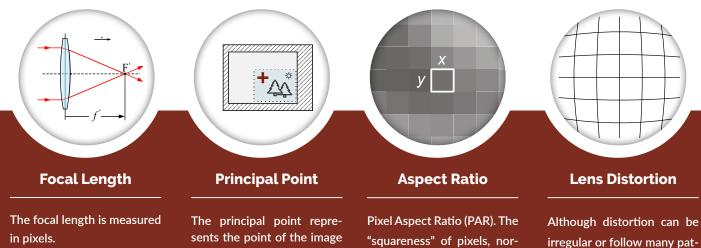
As the focal length varies with focus settings to get the sharpest images in different scenery, the calculated value may differ from the nominal value specified by the lens manufacturer.
