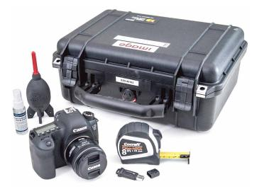
Using the calibrated camera from the system, the operator captures a series of images of a target object or environment to be measured.
